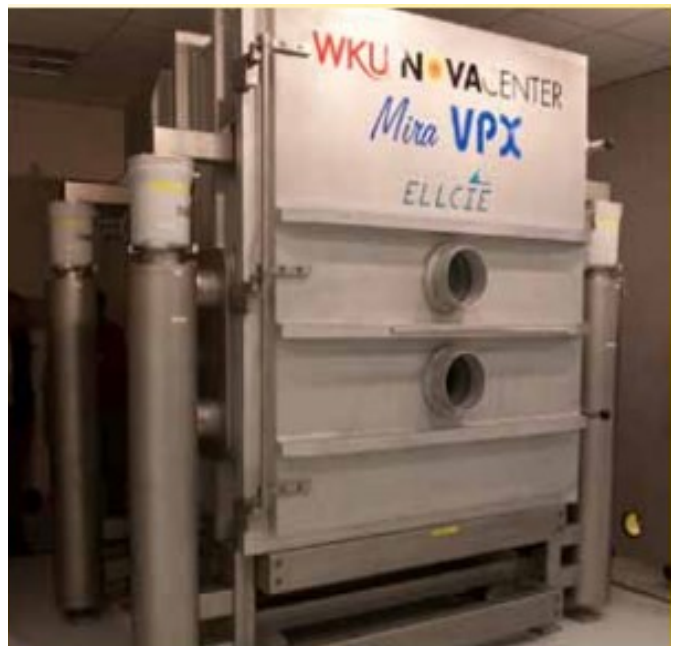
Figure 5. Large-Chamber Scanning Electron Microscope at WKU NOVA Center
